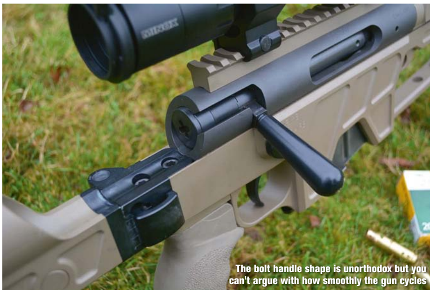
With the bolt remaining below your cheek, you can keep your head welded down for rapid reloads and retained target visibility
